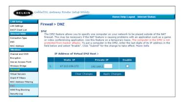
To put a computer in the DMZ, enter the last digits of its IP address in the IP field and select "Enable". Click "Apply Changes" for the change to take effect. If you are using multiple static WAN IP addresses, it is possible to select which WAN IP address the DMZ host will be directed to. Type in the WAN IP address you wish the DMZ host to direct to, enter the last two digits of the IP address of the DMZ host computer, select "Enable" and click "Apply Changes".
